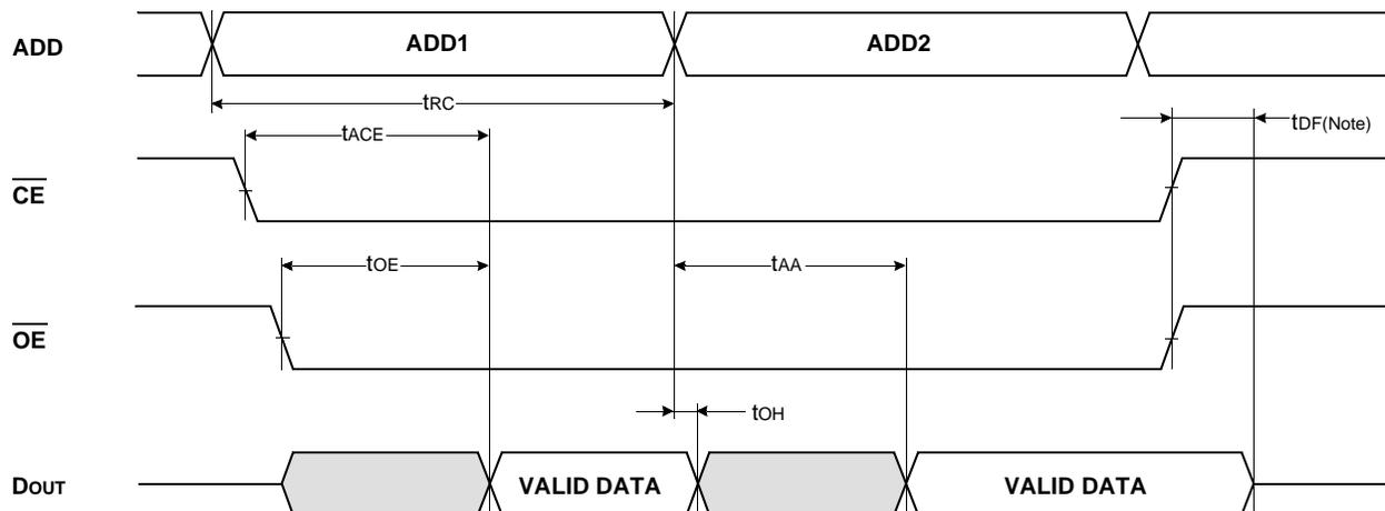
NOTE : t<sub>DF</sub> is defined as the time at which the outputs achieve the open circuit condition and is not referenced to V<sub>OH</sub> or V<sub>OL</sub> level.
