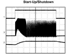
$V_{OUT} = 20V, V_{IN} = 2.5V$ 1) RUN, 1V/div,DC 2)  $V_{OUT}$ , 20V/div,DC 3) I<sub>L</sub>, 200mA/div,DC T=400 $\mu$ s/div R<sub>1</sub>=1.3k $\Omega$
