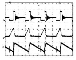
$$\begin{split} V_{\text{OUT}} &= 13.25\text{V}, \ V_{\text{IN}} = 4.2\text{V} \ \text{; 8 LEDs} \\ I_{\text{OUT}} &= 30\text{mA} \\ 1) \ V_{\text{SW}}, \ 20\text{V} \ / \ \text{div}, \ \text{DC} \\ 2) \ \text{Inductor current, 500mA} \ / \ \text{div}, \ \text{DC} \\ 3) \ V_{\text{OUT}}, \ 100\text{mV} \ / \ \text{div}, \ \text{AC} \end{split}$$
