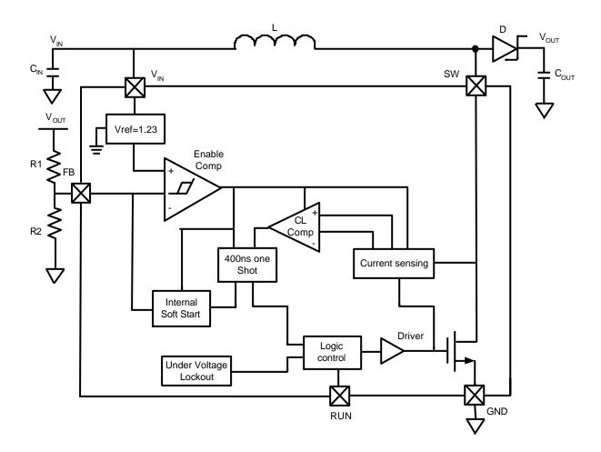
Figure 3: AME5130 Block Diagram
