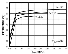
Efficiency vs. Load Current
