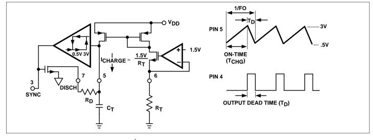
The oscillator frequency (F<sub>O</sub>) =  $\frac{1}{T_{CHG} + T_D}$
