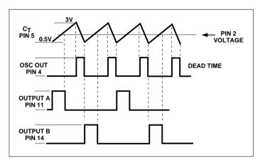
The 5k potentiometer sets a reference voltage at pin 2. When ramp voltage of pin 5 reaches this reference voltage, output drive pulse is active ON. Varying the discharge resistor will vary the dead time. Increasing the discharge resistor will effect an increase in the dead time.
