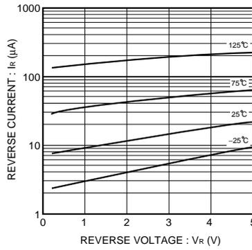
Fig.2 Reverse characteristics
