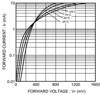
Fig.1 Forward characteristics
