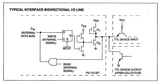
Note: Q1 can be disconnected via mask option to form an "open drain" pin.
