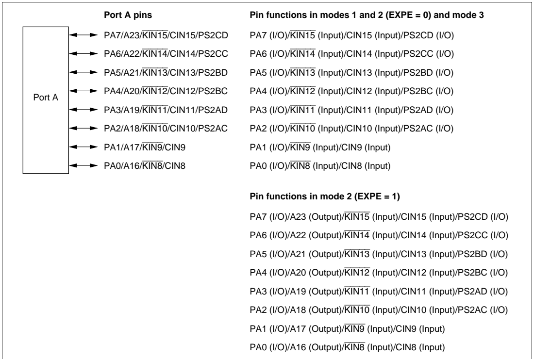
Figure 8.18 Port A Pin Functions
