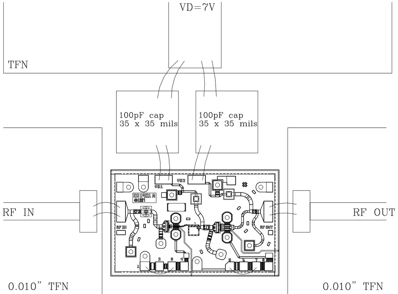
**Chip Assembly and Bonding Diagram**
