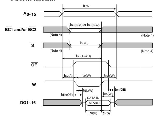
1048576-BIT(65536-WORD BY 16-BIT)CMOS STATIC RAM
