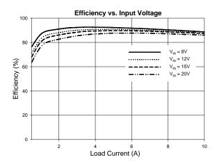
Figure 19. 1.5V PWM Efficiency
