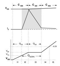
Figure 22. Switching Losses and Q<sub>G</sub>
