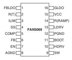
Figure 2. Pin Assignment
