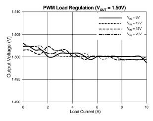
Figure 16. PWM Load Regulation
