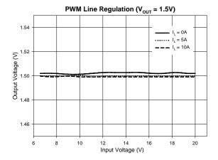
Figure 14. PWM Line Regulation
