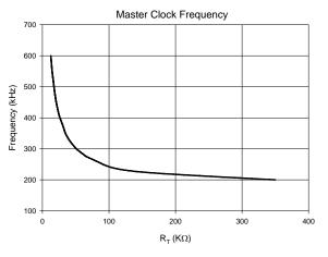
Figure 18. R<sub>T</sub> vs. Frequency
