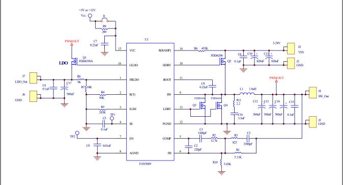
Figure 25. Application Board Schematic
