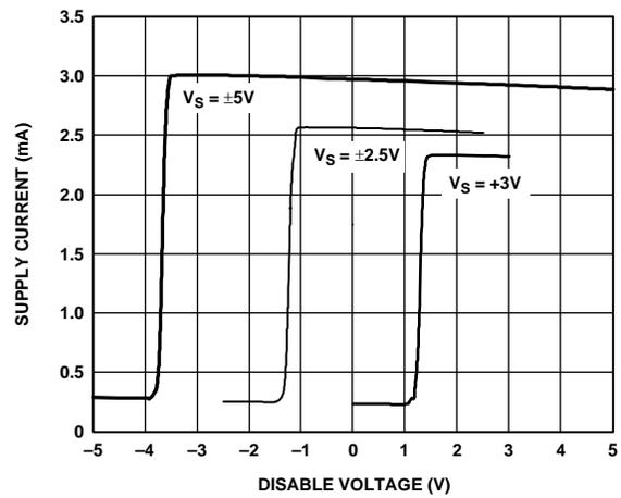
Figure 26. Supply Current vs.  $\overline{\text{POWER DOWN}}$  Pin Voltage
