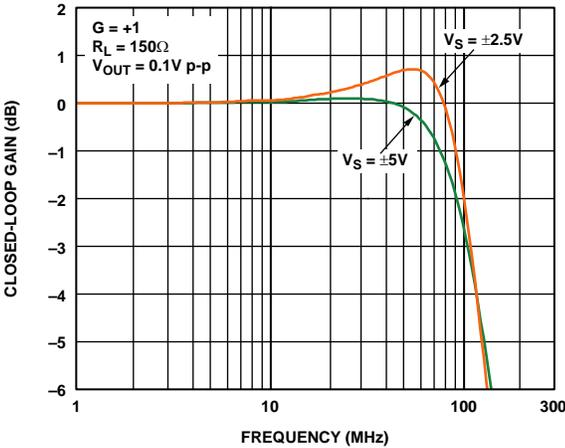
Figure 6. Small Signal Frequency Response for Various Supplies
