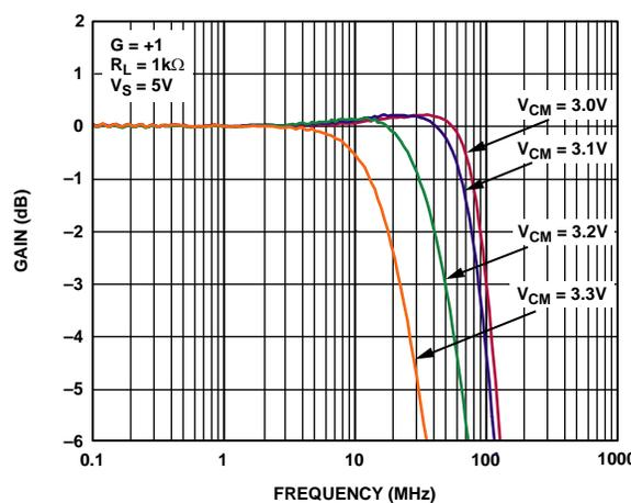
Figure 37. Unity-Gain Follower Bandwidth vs. Input Common-Mode
