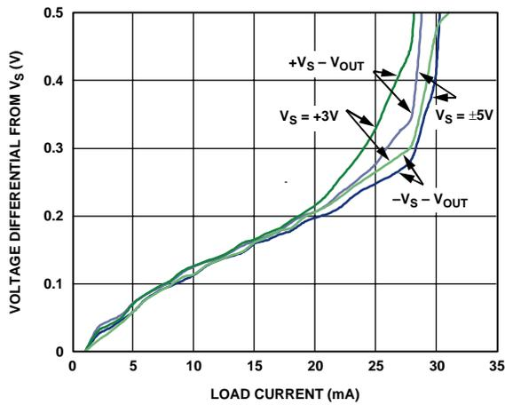
Figure 23. Output Saturation Voltage vs. Load Current
