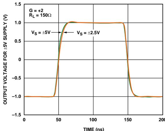
Figure 21. Large Signal Transient Response for Various Supplies
