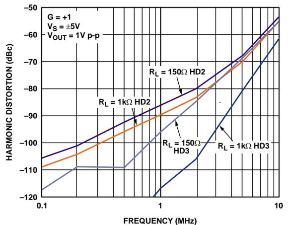
Figure 15. Harmonic Distortion vs. Frequency for Various Loads
