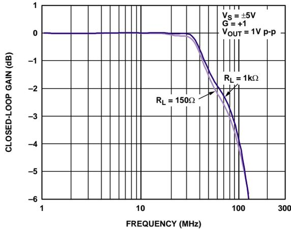
Figure 11. Large Frequency Response for Various Loads
