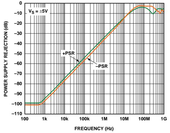
Figure 35. Power Supply Rejection (PSR) vs. Frequency
