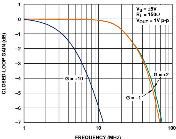
Figure 9. Large Signal Frequency Response for Various Gains
