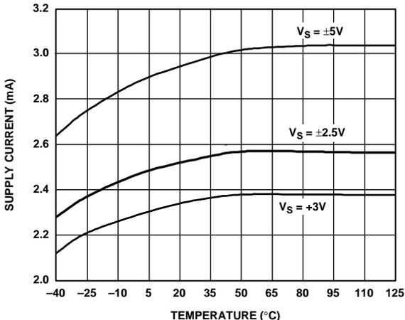
Figure 30. Supply Current vs. Temperature for Various Supplies
