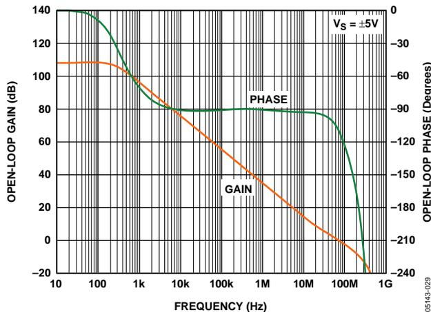
Figure 12. Open-Loop Gain and Phase vs. Frequency
