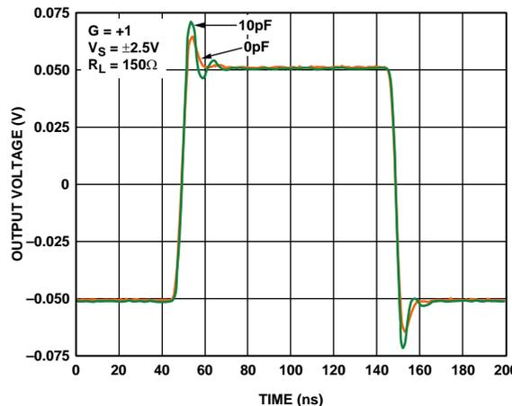
Figure 20. Small Signal Transient Response for Capacitive Load
