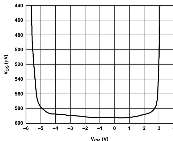
Figure 36.  $V_{OS}$  vs. Common-Mode Voltage,  $V_S = \pm 5$  V
