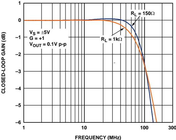
Figure 5. Small Signal Frequency Response for Various Loads
