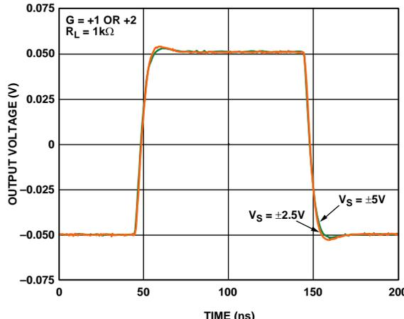
Figure 19. Small Signal Transient Response for Various Supplies
