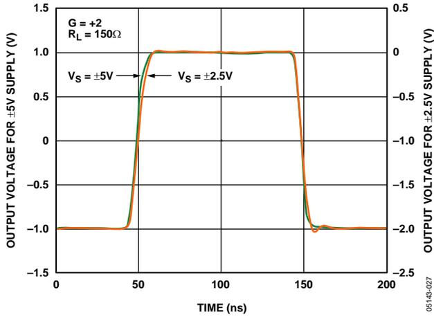
Figure 22. Large Signal Transient Response for Various Supplies
