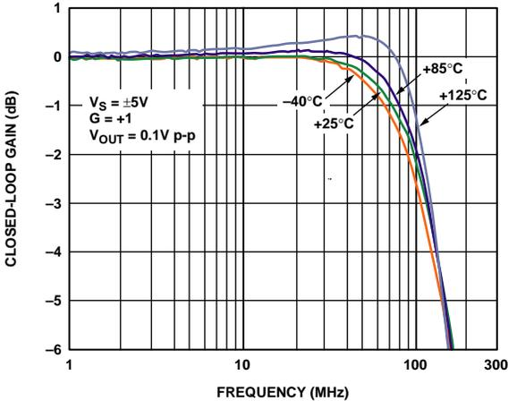
Figure 8. Small Signal Frequency Response for Various Temperatures
