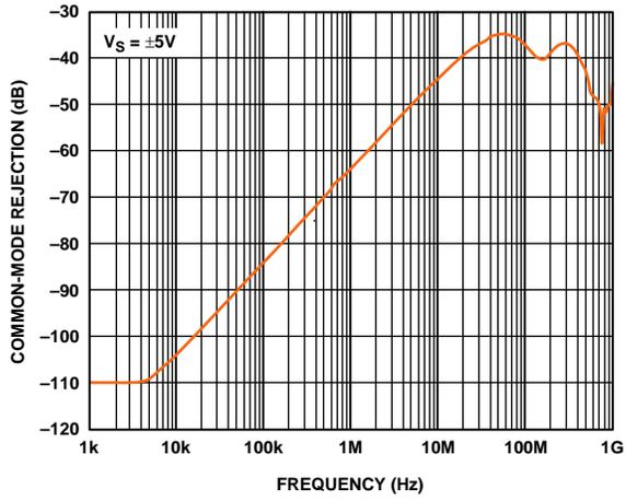
Figure 34. Common-Mode Rejection Ratio (CMRR) vs. Frequency
