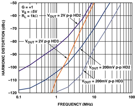
Figure 16. Harmonic Distortion vs. Frequency for Various  $V_{OUT}$
