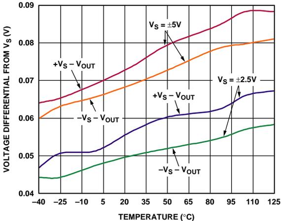
Figure 29. Output Saturation vs. Temperature for Various Supplies
