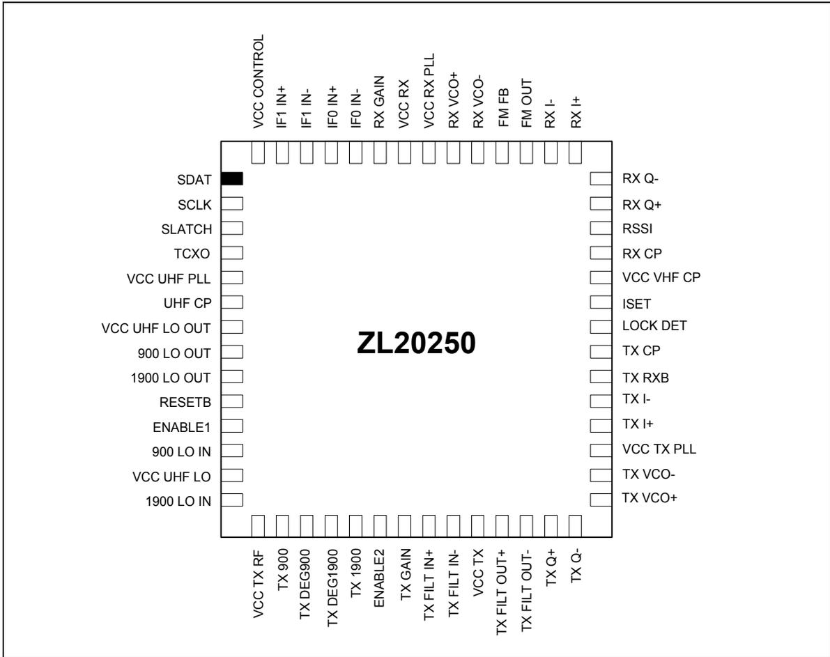
Figure 2 - ZL20250 Package Diagram
