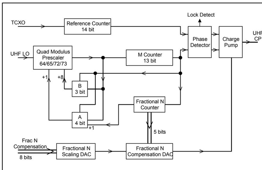
Figure 9 - UHF Synthesizer
