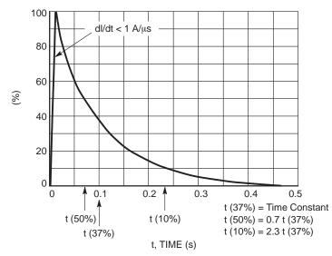
Figure 12. Load Dump Pulse Current
