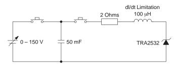
Figure 11. Load Dump Test Circuit
