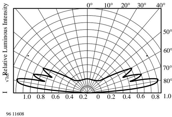
Figure 4 Rel. Luminous Intensity vs. Angular Displacement
