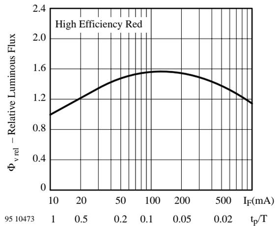
Figure 7 Rel. Luminous Flux vs. Forw. Current/Duty Cycle
