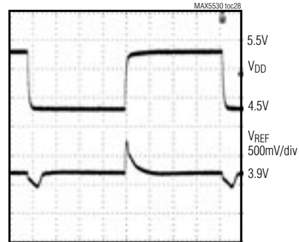
REFERENCE LINE-TRANSIENT RESPONSE ( V_{REF} = 3.9V )
