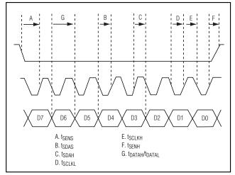
Figure 1. Serial-Interface Timing Diagram
