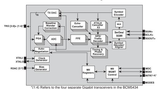
The **BCM5434** consists of four complete 10/100/1000BASE-T Gigabit Ethernet transceivers integrated on a single monolithic CMOS chip. The **BCM5434** is optimized for low power and small footprint size to enable high port density applications. By doubling transceiver port density,
