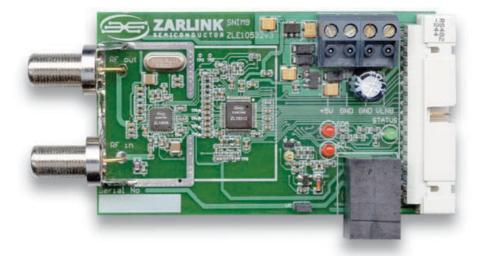
The ZLE10532 is a complete front-end reference design for reception of digital satellite TV signals. This reference design takes advantage of Zarlink's highly integrated satellite front-end chipset, which includes the ZL10036 Zero IF (ZIF) tuner and ZL10312 QPSK demodulator.
