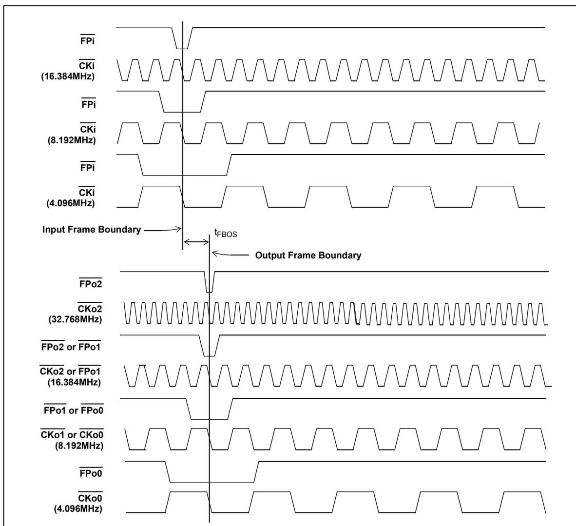
**Figure 39 - Input and Output Frame Boundary Offset**
