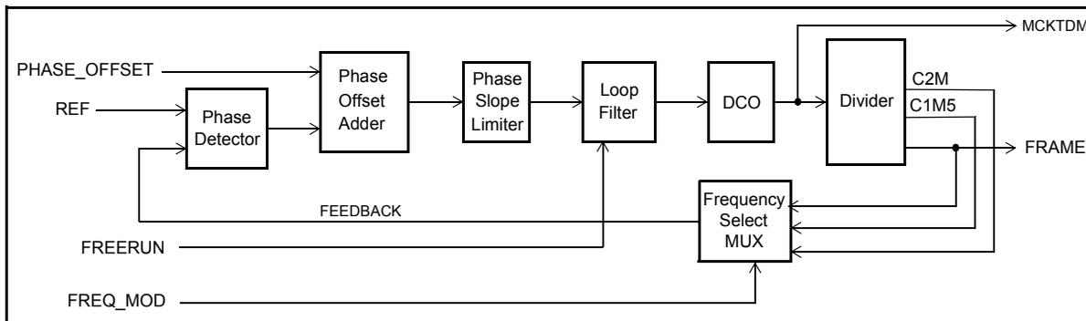
**Figure 27 - Block Diagram of the PLL Module**
