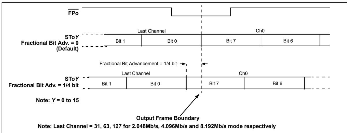
Figure 19 - Fractional Output Bit Advancement Timing Diagram
