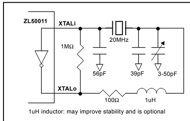
**Figure 30 - Crystal Oscillator Circuit**
