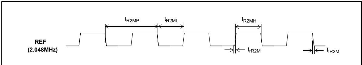
**Figure 37 - Reference Input Timing Diagram when the input frequency = 2.048MHz**
