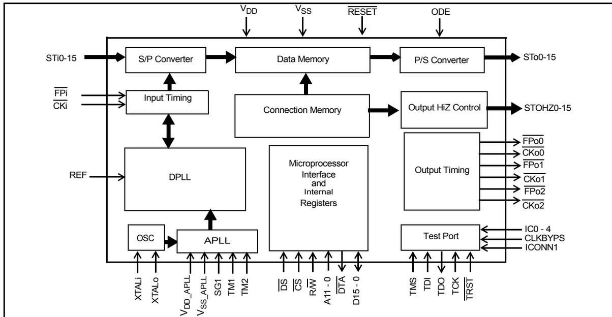
**Figure 1 - ZL50011 Functional Block Diagram**
