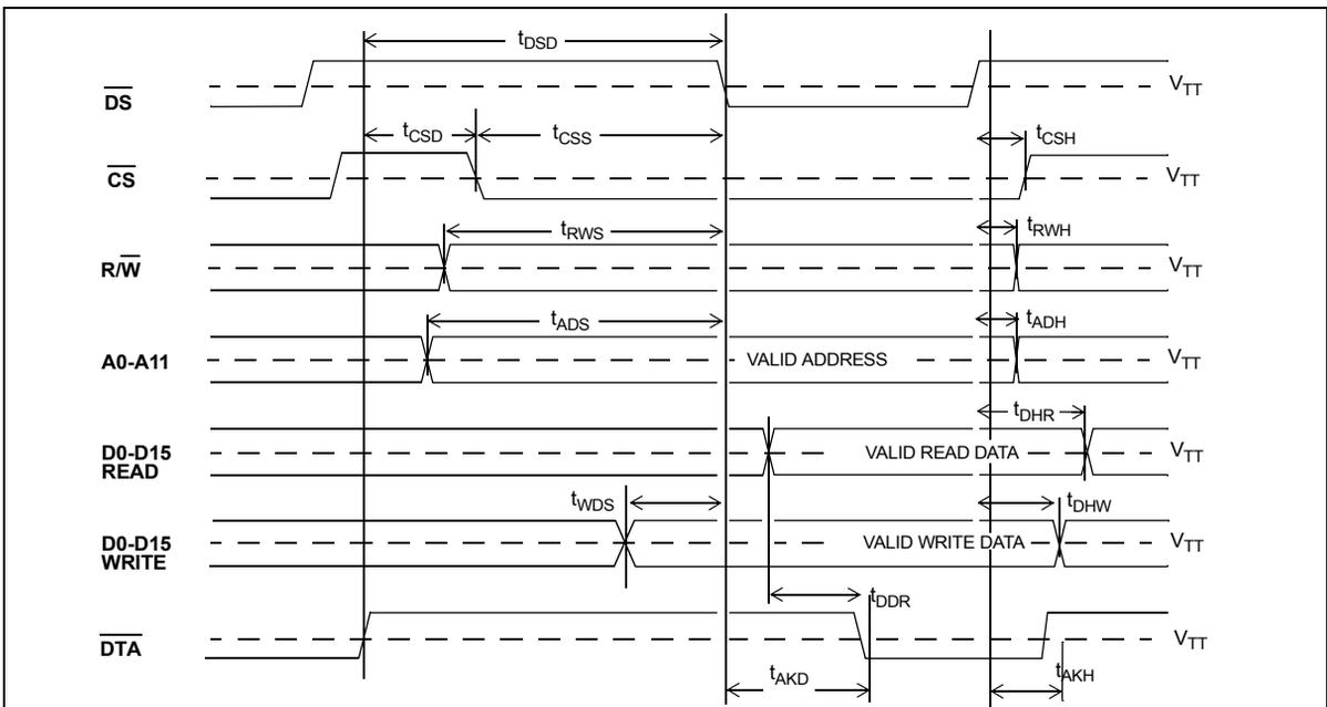
Figure 47 - Motorola Non-Multiplexed Bus Timing
