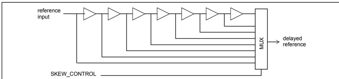
Figure 26 - Skew Control Circuit Diagram
