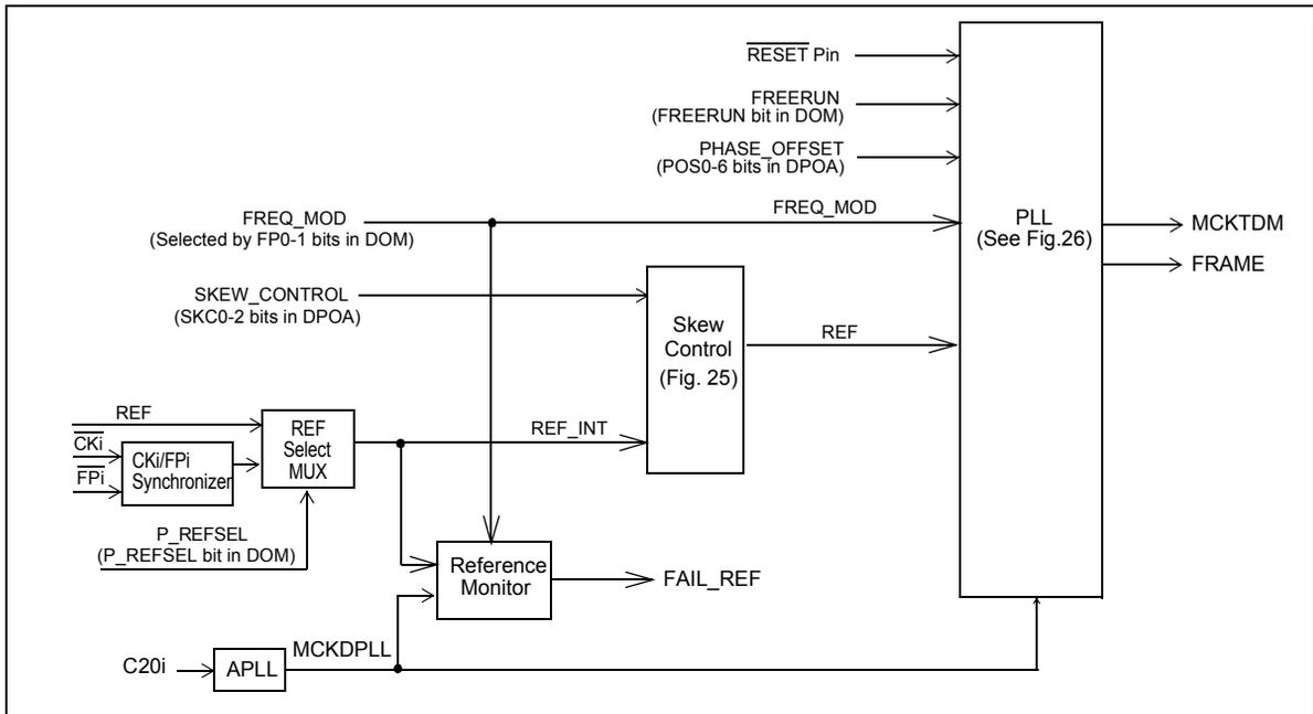
Figure 25 - DPLL Functional Block Diagram
