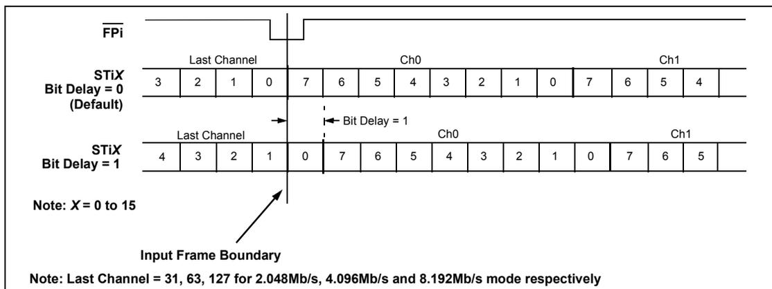
Figure 16 - Input Bit Delay Timing Diagram
