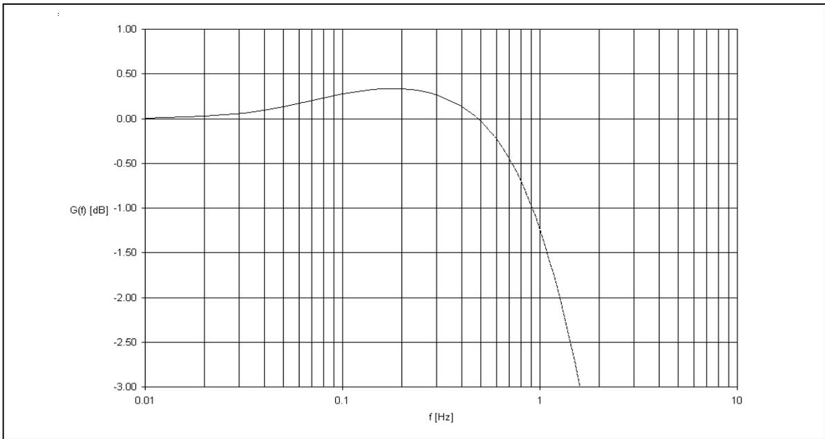
**Figure 29 - Detailed DPLL Jitter Transfer Function Diagram (Wander Transfer Diagram)**
