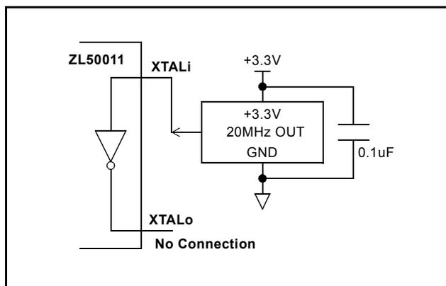
Figure 31 - External Clock Oscillator Circuit
