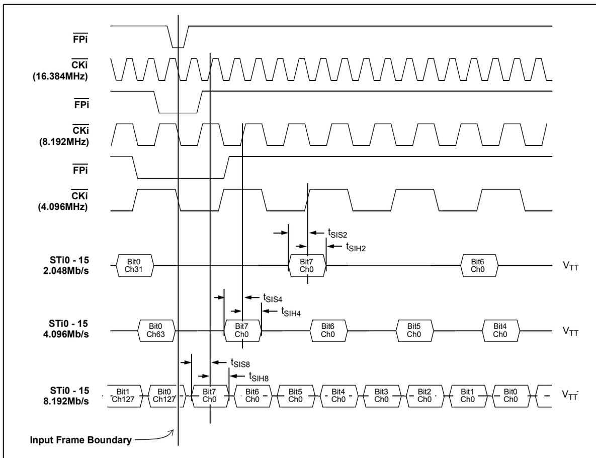
Figure 43 - ST-BUS Inputs (STi0 - 15) Timing Diagram
