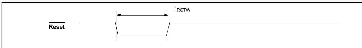
Figure 49 - Reset Pin Timing Diagram
