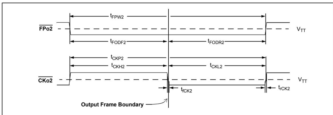
**Figure 42 -  $\overline{\text{FPo2}}$  and  $\overline{\text{CKo2}}$  Timing Diagram**
