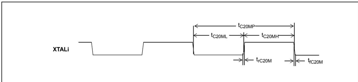
**Figure 35 - XTALi Input Timing Diagram when Clock Oscillator is connected**
