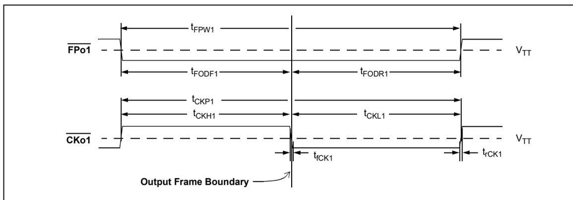
**Figure 41 -  $\overline{FPo1}$  and  $\overline{CKo1}$  Timing Diagram**
