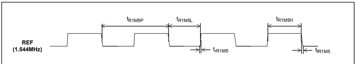
**Figure 38 - Reference Input Timing Diagram when the input frequency = 1.544Hz**
