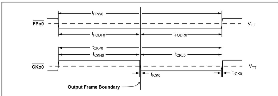
**Figure 40 -  $\overline{\text{FPo0}}$  and  $\overline{\text{CKo0}}$  Timing Diagram**
