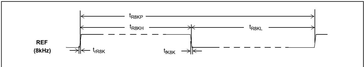
**Figure 36 - Reference Input Timing Diagram when the input frequency = 8kHz**
