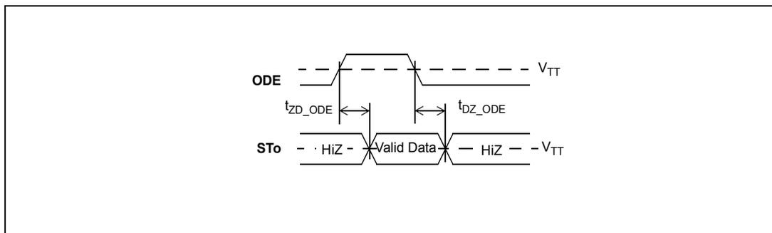
**Figure 46 - Output Driver Enable (ODE)**
