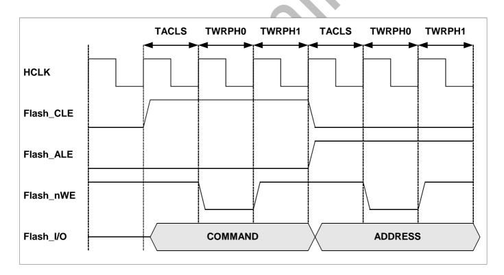
Figure 4-4 Auto Mode Timing Diagram (TACLS = 1, TWRPH0 = 0, TWRPH1 = 0)
