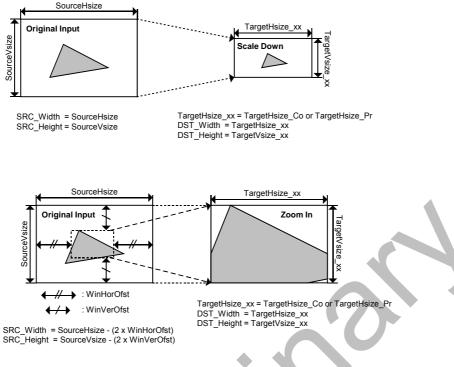
Figure 21-15 Scaling scheme
