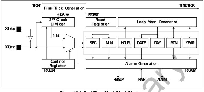
Figure 10-1. Real Time Clock Block Diagram
