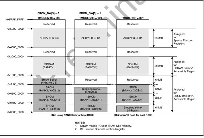
Figure 2-1. SROM Controller Address Mapping
