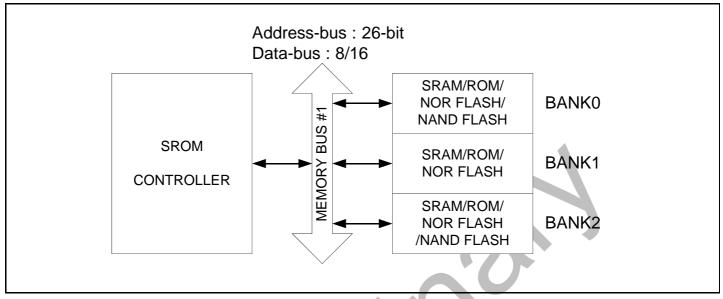
Figure 2-3 Memory Interface Block Diagram
