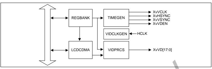
Figure 28-1. LCD Controller Block Diagram
