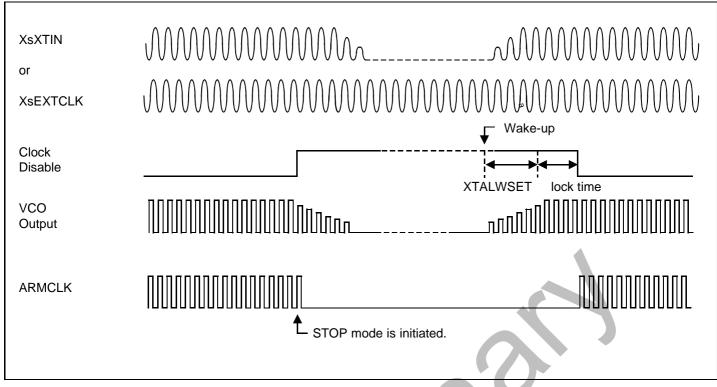
Figure 33-6. Entering STOP Mode and Exiting STOP mode (Wake-up)
