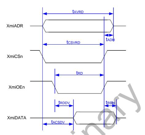
Figure 19-4 Modem interface read timing diagram
