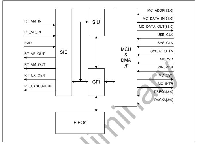
Figure 18-1. USB Device Block Diagram
