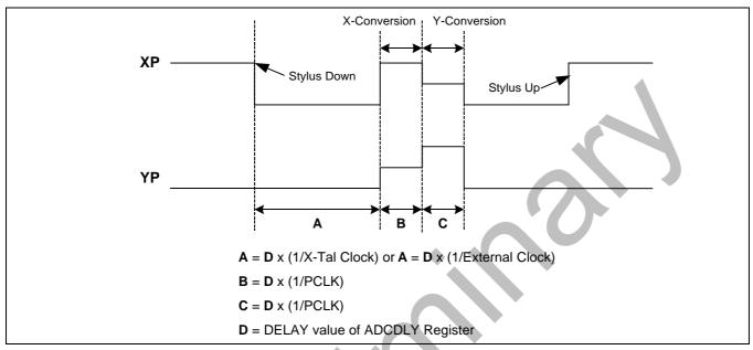
Figure 30-3 Timing Diagram at Auto (Sequential) X/Y Position Conversion Mode
