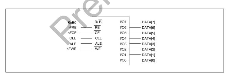
Figure 4-7 8-bit NAND Flash Memory Interface
