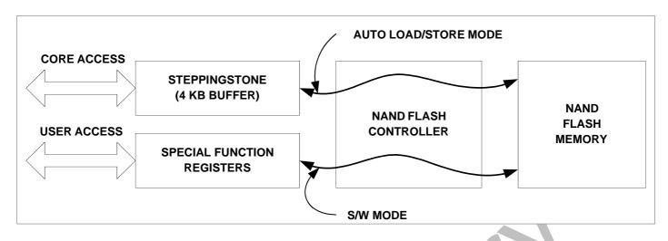
Figure 4-3 NAND Flash Controller Operation Mode Block Diagram
