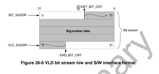
S/W must be set BIT\_SADDR and START\_BIT\_CNT and bitstream data. BIT\_SADDR is address of start coefficient bit stream. And START\_BIT\_CNT is start bit of current macro block bit stream. And bitstream data must be big-endian data. VLD h/w generate VLC\_EADDR and END\_BIT\_CNT value after macro block VLD operation. Before next macro block start s/w have to find BIT\_SADDR and START\_BIT\_CNT after header parsing and VLD.
