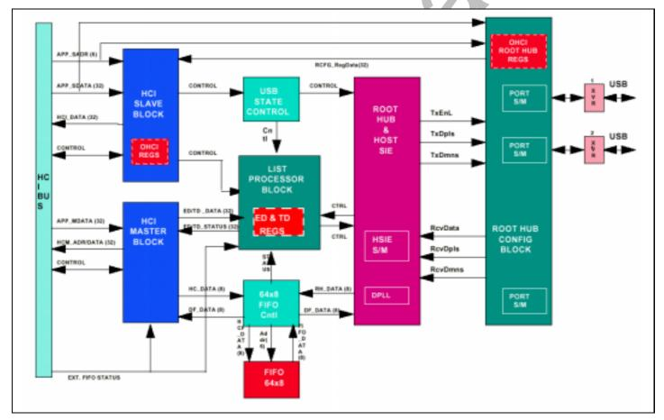
Figure 17-1. USB Host Controller Block Diagram
