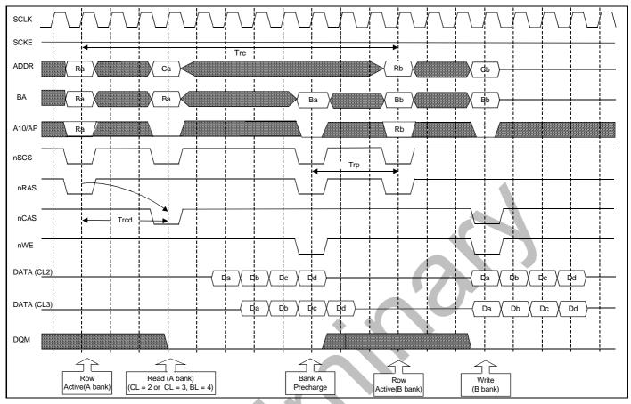
Figure 3-3. SDRAM Timing Diagram
