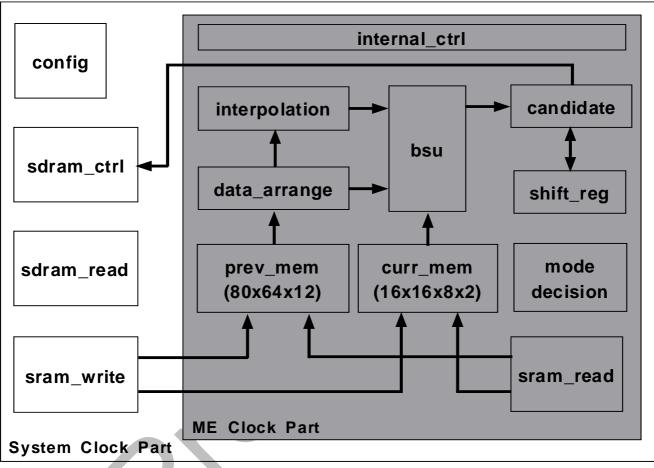
Figure 23-1. MPEG-4 Motion Estimation Block Diagram
