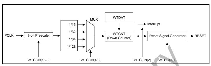
Figure 8-1. Watchdog Timer Block Diagram
