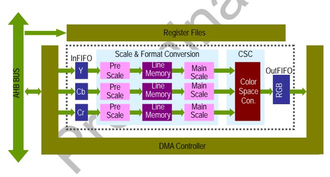
Figure 27-1. Block Diagram of Post Processor
