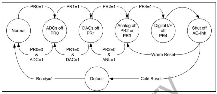
Figure 16-8 AC97 Power down/Power up Flow
