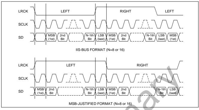
Figure 14-2. IIS-Bus and MSB(Left)-justified Data Interface Formats
