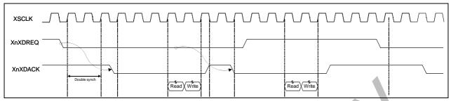
Figure 9-4. Single service, Demand Mode, Single Transfer Size
