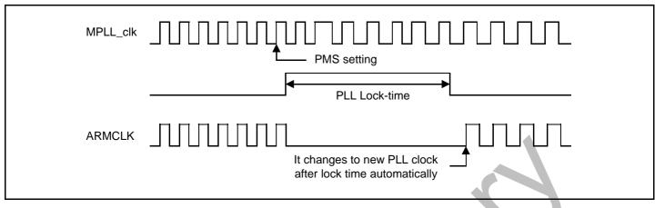
Figure 33-4. The case that changes Slow clock by setting PMS value
