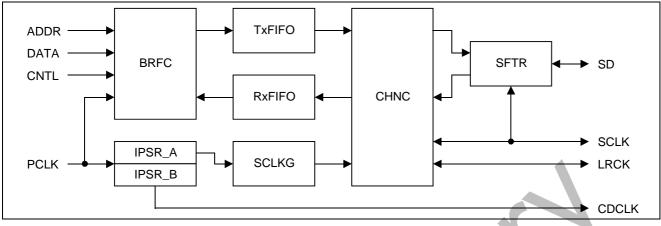
Figure 14-1. IIS-Bus Block Diagram
