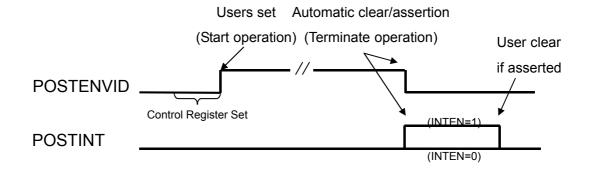
Figure 27-8 Start and termination of the operation of POST PROCESSOR
