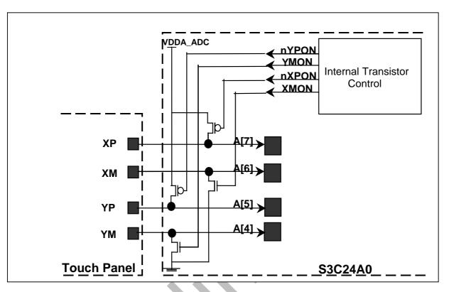
Figure 30-2. Example of ADC and Touch Screen Interface
