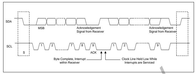
Figure 13-4. Data Transfer on the IIC-Bus
