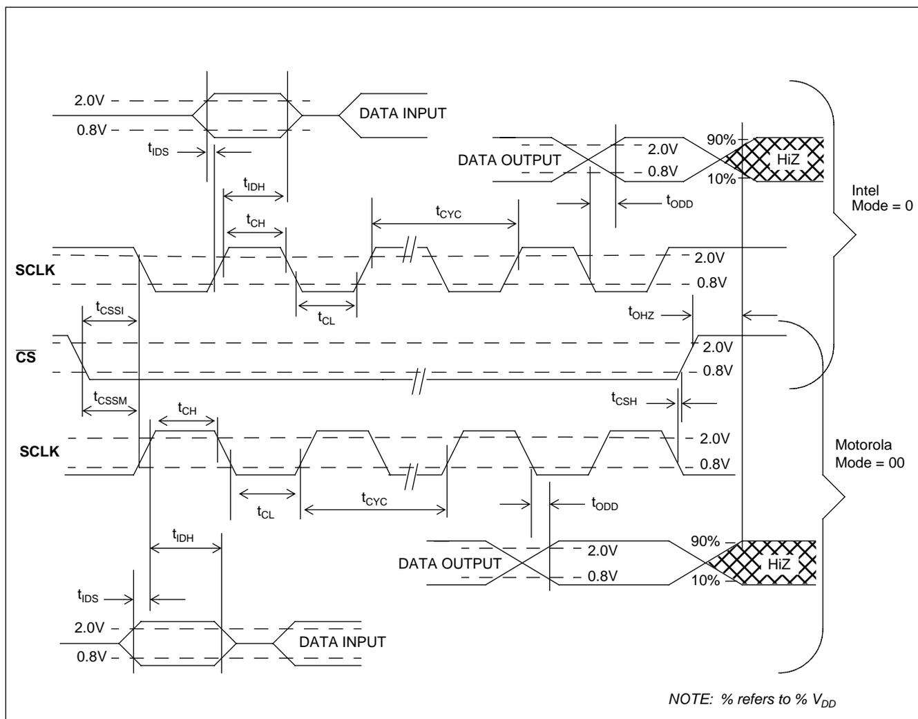
Figure 14 - Microport Timing
