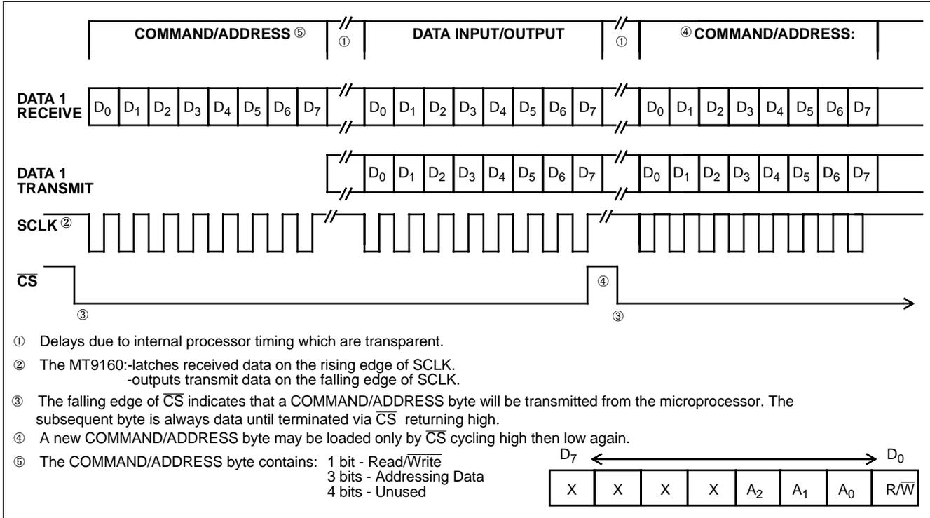
**Figure 4 - Serial Port Relative Timing for Intel Mode 0**
