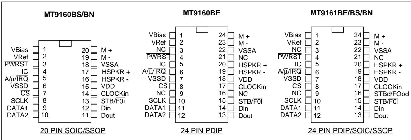
Figure 2 - Pin Connections
