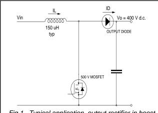
Fig.1. Typical application, output rectifier in boost converter power factor correction circuit. Continuous conduction, mode where the transistor turns on whilst forward current is still flowing in the diode.
