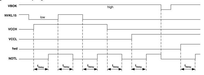
Figure 6. Push-pull Output NOTL
