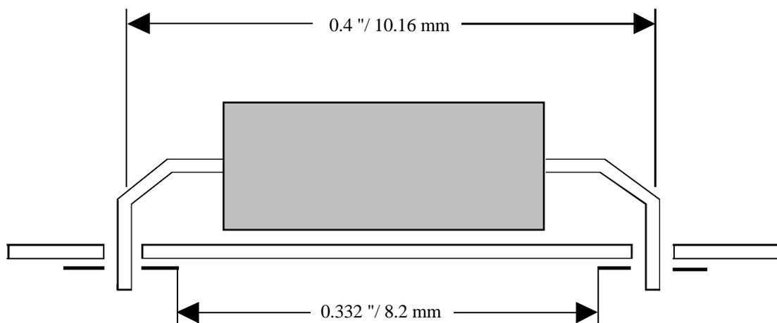
Figure 2. Optocoupler mounting on a board (side view)
