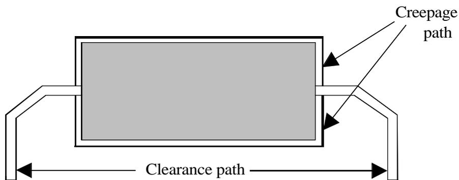
Figure 1. Isolation creepage/ clearance path
