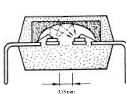
Figure 4. Cut through of a TEMIC optocoupler (thickness through insulation)
