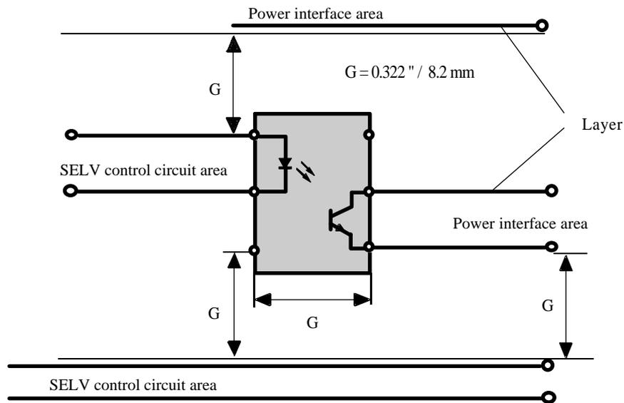
Figure 3. Top view of optocoupler mounting on a board
