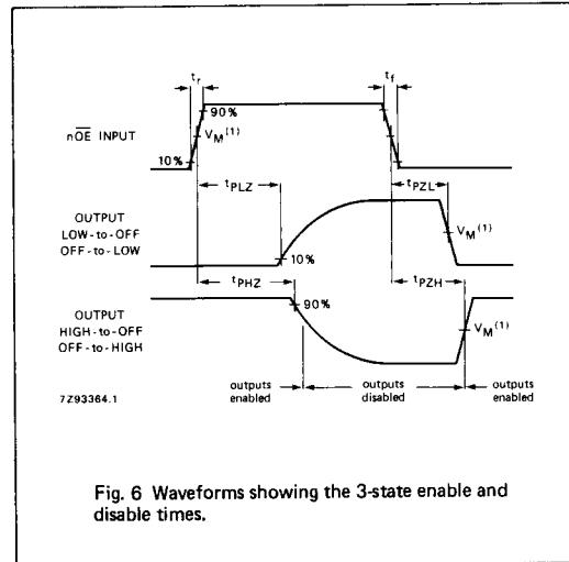
Fig. 6 Waveforms showing the 3-state enable and disable times.
