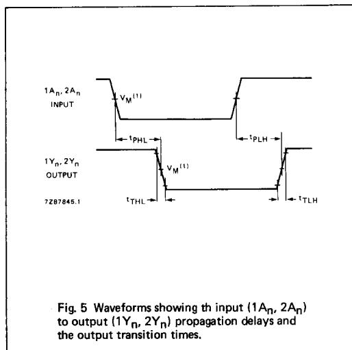
Fig. 5 Waveforms showing th input ( $1A_n, 2A_n$ ) to output ( $1Y_n, 2Y_n$ ) propagation delays and the output transition times.
