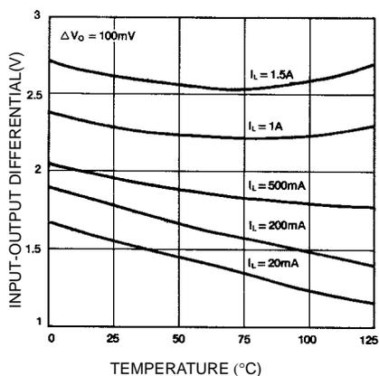
Figure 3. Dropout Voltage
