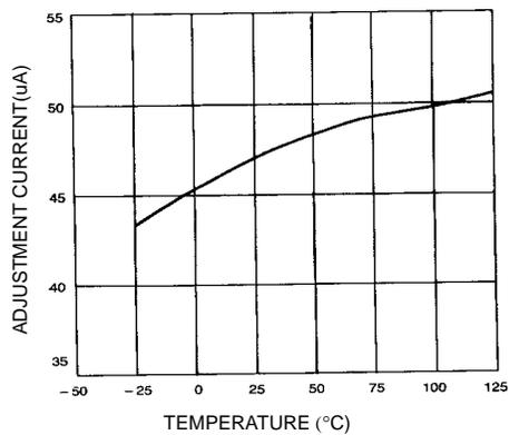
Figure 2. Adjustment Current
