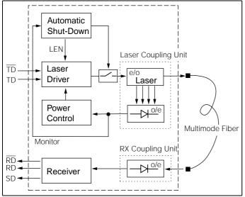
The receiver component converts the optical serial data into PECL compatible electrical data (RD and RDnot) which are AC coupled with a biasing build into the transceiver. The Signal Detect (SD, active high) shows whether an optical signal is present.
