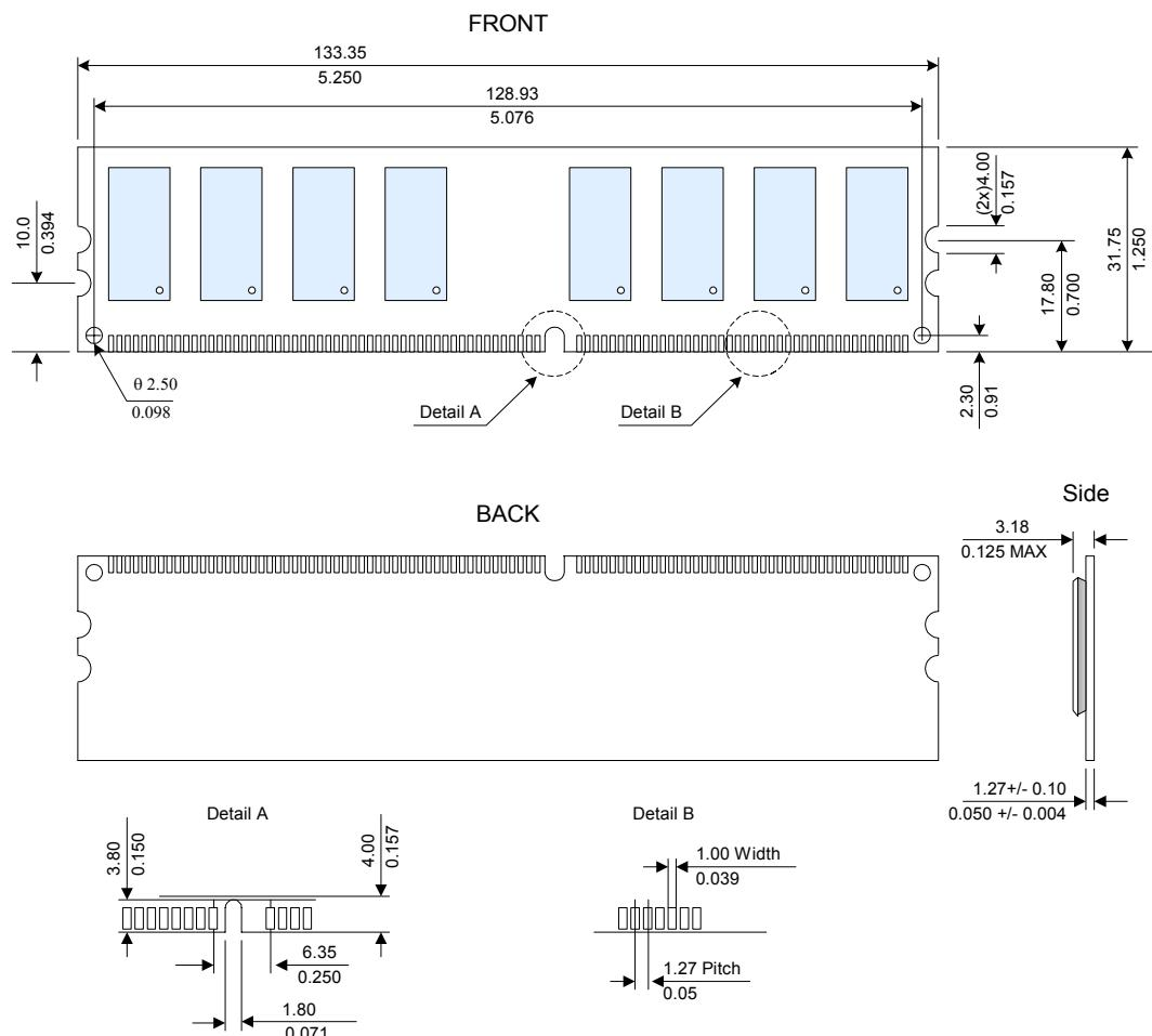
Note: All dimensions are typical with tolerances of +/- 0.15 (0.006) unless otherwise stated.
