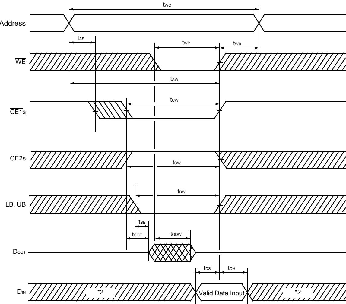
\*1 : If  $\overline{\text{OE}}$  is HIGH during the write cycle, the outputs will remain at high impedance.
