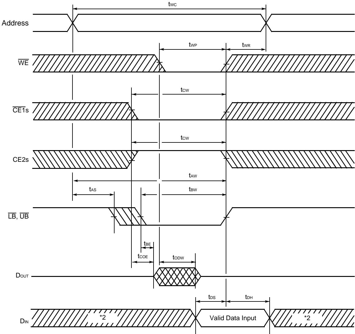
\*1 : If OE is HIGH during the write cycle, the outputs will remain at high impedance.
