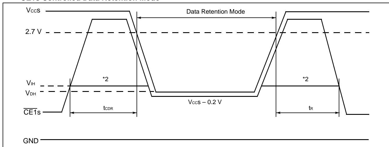
\*1 : In  $\overline{CE1s}$  controlled data retention mode, input level of  $CE2s$  should be fixed  $V_{CCS}$  to  $V_{CCS}-0.2 \text{ V}$  or  $V_{SS}$  to  $0.2 \text{ V}$  during data retention mode. Other input and input/output pins can be used between  $-0.3 \text{ V}$  to  $V_{CCS}+0.3 \text{ V}$ .
