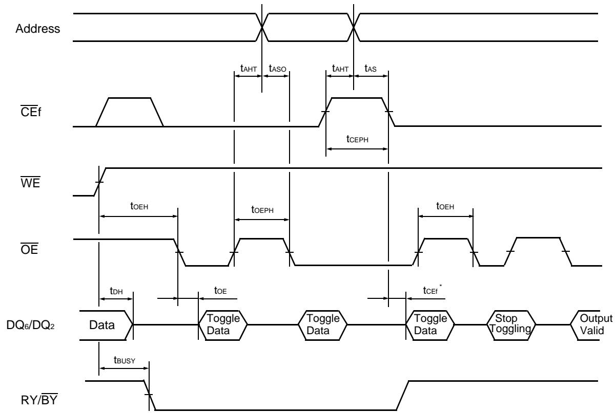
\* :  $DQ_6$  stops toggling (The device has completed the Embedded operation).
