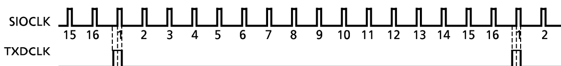
Figure 3.11 (14) Generation of Transmission Clock
