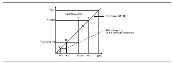
The buffer OP-amp selects the lower command between  $V_{CMD}$  and  $V_{La}$  so as to limit the stalled motor current to very low in the above figure. Because of much larger  $V_{La}$  than  $V_{CMD}$ , the motor operating point stays at A. But the point gradually moves toward B' and then B" through the curve from the instance of stall as the below figure.
