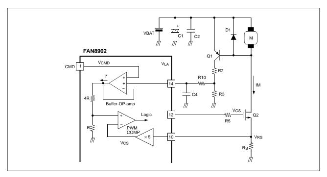
In the steady state, the terminal voltage on a motor is consisted of a back EMF and the voltage drop on the armarture resistors. When the motor happens to be stalled, the back EMF becomes zero, and the motor current  $(I_M)$  is quickly increased until a maximum values.
