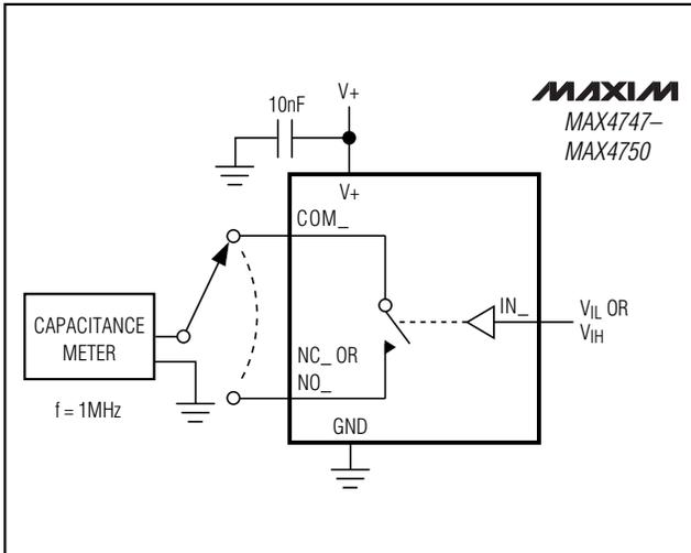
Figure 7. Channel Off/On-Capacitance
