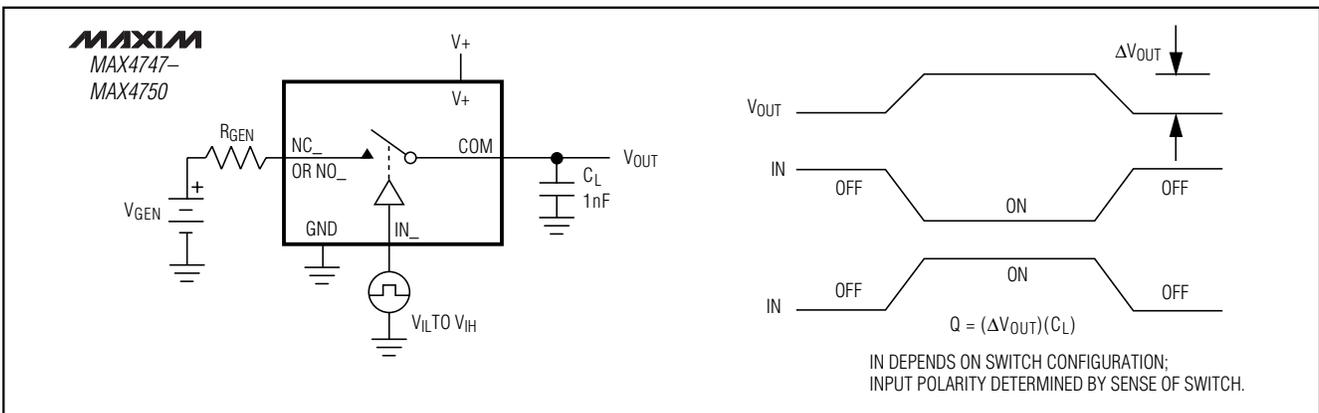
Figure 4. Charge Injection
