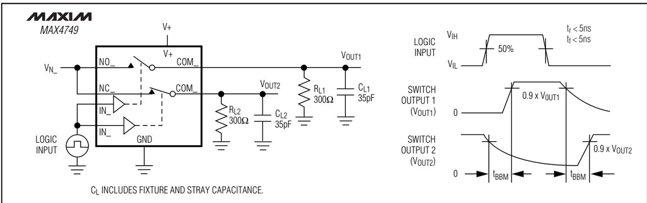
Figure 3. Break-Before-Make Interval
