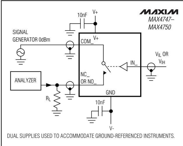
Figure 5. Off-Isolation/On-Channel Bandwidth
