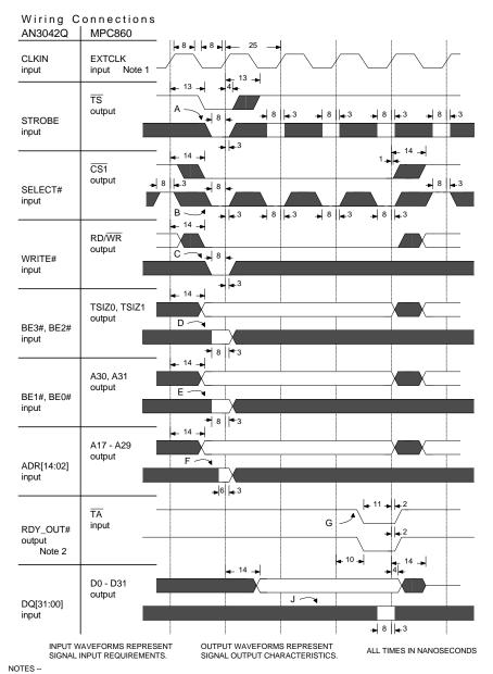
1 MPC860 bus interface timing is related to its CLKOUT signal output. A phase lock loop within the MPC860 keeps the phase skew between its EXTCLK input and CLKOUT output at + 0.9 nsec. That value is factored into this timing diagram. The minimum high and low times for the AN3042Q CLKIN input are shown.
