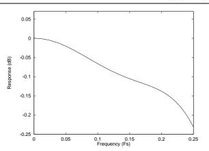
Figure 27 DAC Digital Filter Frequency Response-Type 3
