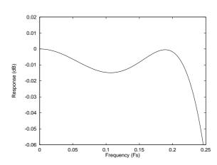
Figure 25 DAC Digital Filter Frequency Response-Type 2
