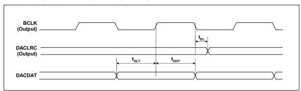
Figure 2 Digital Audio Data Timing - Master Mode
