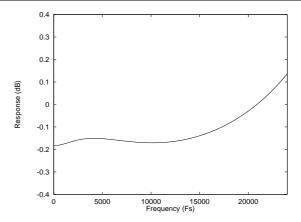
Figure 33 De-Emphasis Frequency Response (48kHz)
