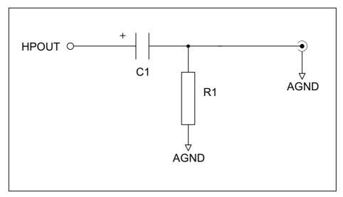
Figure 11 Headphone Output Application Drawing
