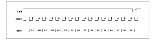
Figure 19 3-Wire Serial Interface
