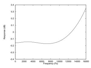
Figure 29 De-Emphasis Frequency Response (32kHz)
