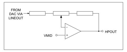
Figure 10 Headphone Amplifier Schematic
