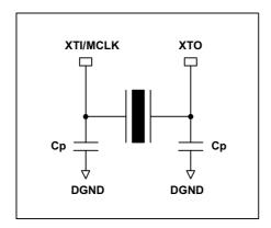
Figure 12 Crystal Oscillator Application Circuit
