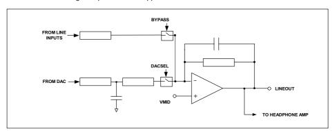
Figure 8 Line Output Schematic
