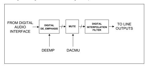
Figure 6 DAC Filter Schematic
