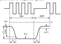
Tr: Time for segment to darken 90% after selective waveform switches to non-selective waveform.
