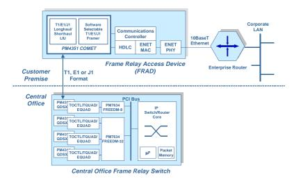
Figure 4: Frame Relay Access Device (FRAD) using COMET
