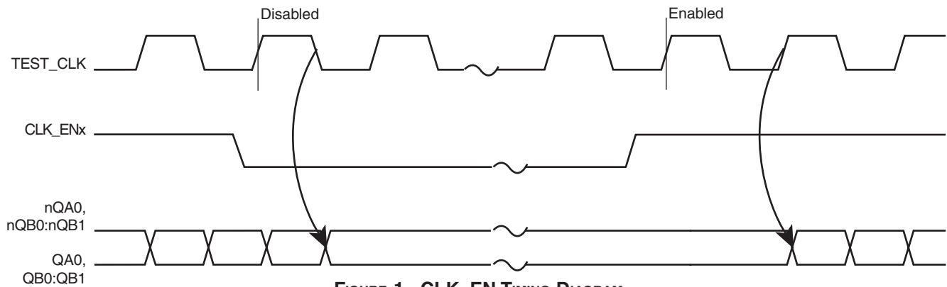
FIGURE 1. CLK_EN TIMING DIAGRAM
