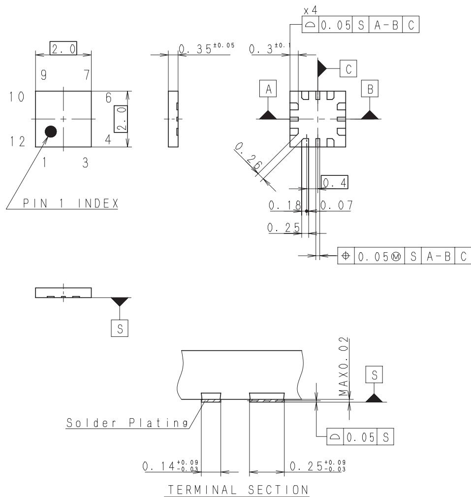
Note: Cutting burr of lead are 0.05mm MAX.
