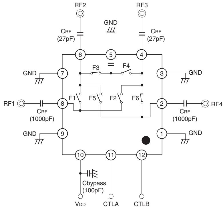
When using this IC, the following external components should be used:
