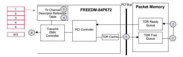
For this analysis, it is assumed that the transmit packets are composed of a single descriptor or buffer. Linking of multiple descriptors to form a packet involves additional overhead activity on the PCI bus.
