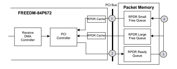
For this analysis, it is assumed that the receive packets are composed of a single descriptor or buffer. Linking of multiple descriptors to form a packet involves additional overhead activity on the PCI bus.
