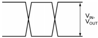
Figure 5a. Single-Ended Voltage Swing
