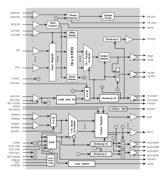
The BCM8212 SONET/SDH transceiver is a fully integrated serialization/deserialization SONET OC-48 (2.488 Gbps) interface device with an integrated Clock Multiplication Unit (CMU) and an integrated Clock and Data Recovery (CDR) circuit. On-chip clock synthesis is performed by the high-frequency and low-jitter, phaselocked loop on the BCM8212 transceiver chip, allowing the use of a slower 77.76/155.52-MHz external transmit clock reference.
