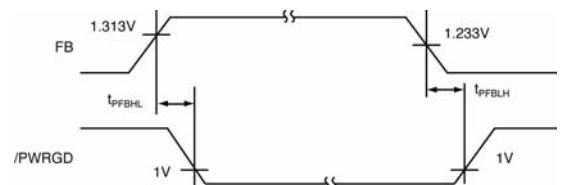
Figure 4. MIC2587/87R-2 FB to /PWRGD Timing
