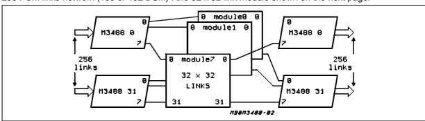
2048 PCM links network (1792 or 2048 DSM): the 256 x 256 link network is shown above.
