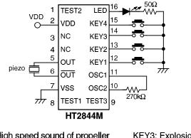
KEY1: High speed sound of propellerKEY3: ExplosionKEY2: Low speed sound of propellerKEY4: Machine Gun
