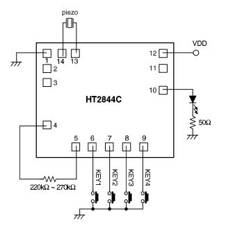
\* The IC substrate should be connected to VDD in the PCB layout artwork.
