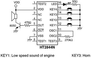
KEY2: High speed sound of engine KEY4: Brake
