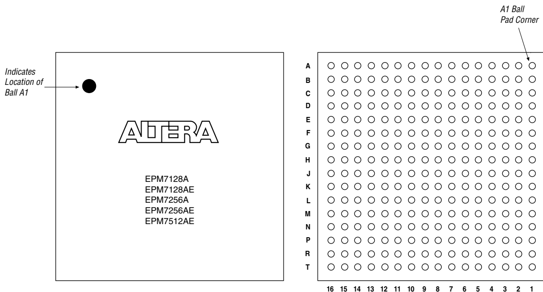
Figure 23. 256-Pin FineLine BGA Package Pin-Out Diagram
