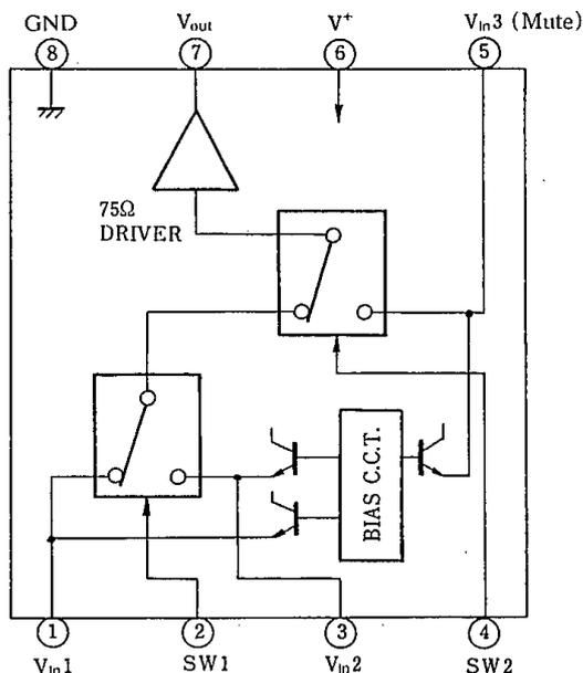
■ INPUT CONTROL SIGNAL-OUTPUT SIGNAL
