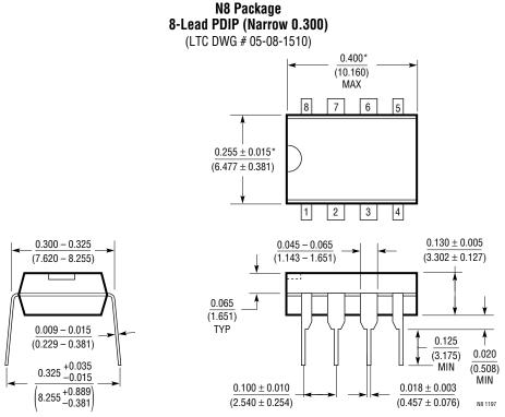
\*THESE DIMENSIONS DO NOT INCLUDE MOLD FLASH OR PROTRUSIONS. MOLD FLASH OR PROTRUSIONS SHALL NOT EXCEED 0.010 INCH (0.254mm)
