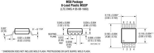
PROTRUSIONS OR GATE BURRS SHALL NOT EXCEED 0.006" (0.152mm) PER SIDE DIMENSION DOES NOT INCLUDE INTERLEAD FLASH OR PROTRUSIONS.
