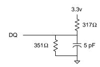
Fig. 2 OUTPUT LOAD EQUIVALENT
