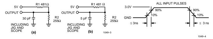
Equivalent to: THÉVENIN EQUIVALENT \_\_\_\_\_O 1.73V
