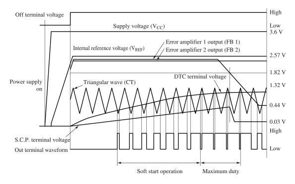
2. Short-circuit protection operation waveform
