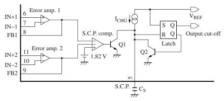
Figure 4. Short-circuit protection circuit
