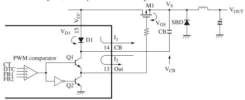
Figure 6. Output block and bootstrap circuit
