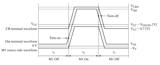
Figure 7. Bootstrap circuit operation waveform
