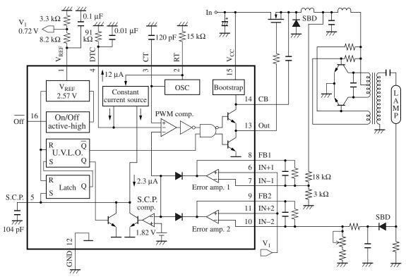
• DC-DC converter control (step-up circuit example)
