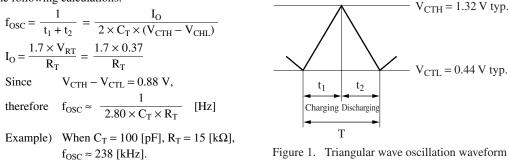
It is possible to use the circuit in the recommended operating range of 5 kHz to 500 kHz of the oscillation frequency. In addition, when the oscillation frequency becomes high, overshoot and undershoot are generated due to the operation delay of the triangular oscillation comparator. Care should be taken because the actual measurement values deviate from the above calculation values.
