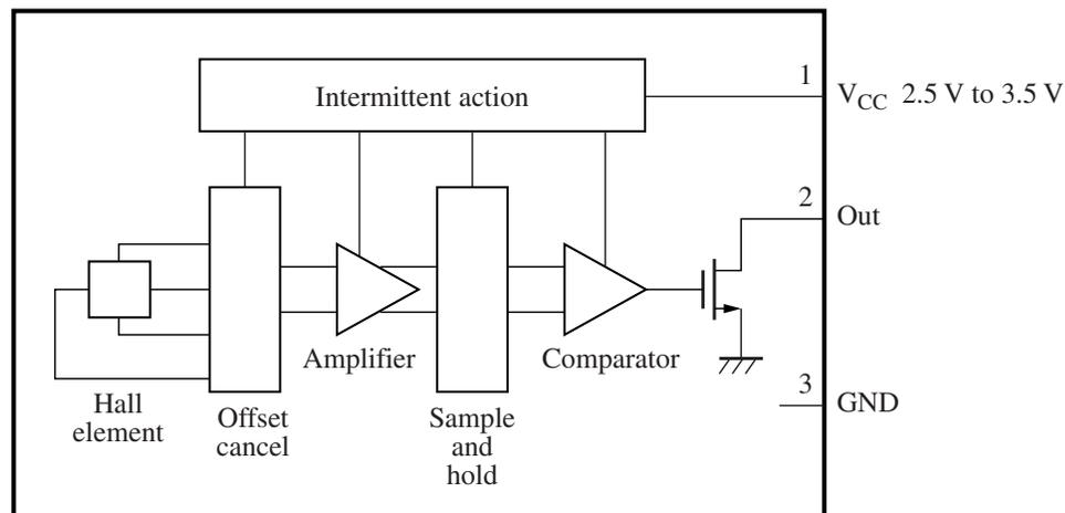
Note) The magnetism detection time should be longer than one intermittent action cycle (On = 200  $\mu$ s and Off = 51 ms).
